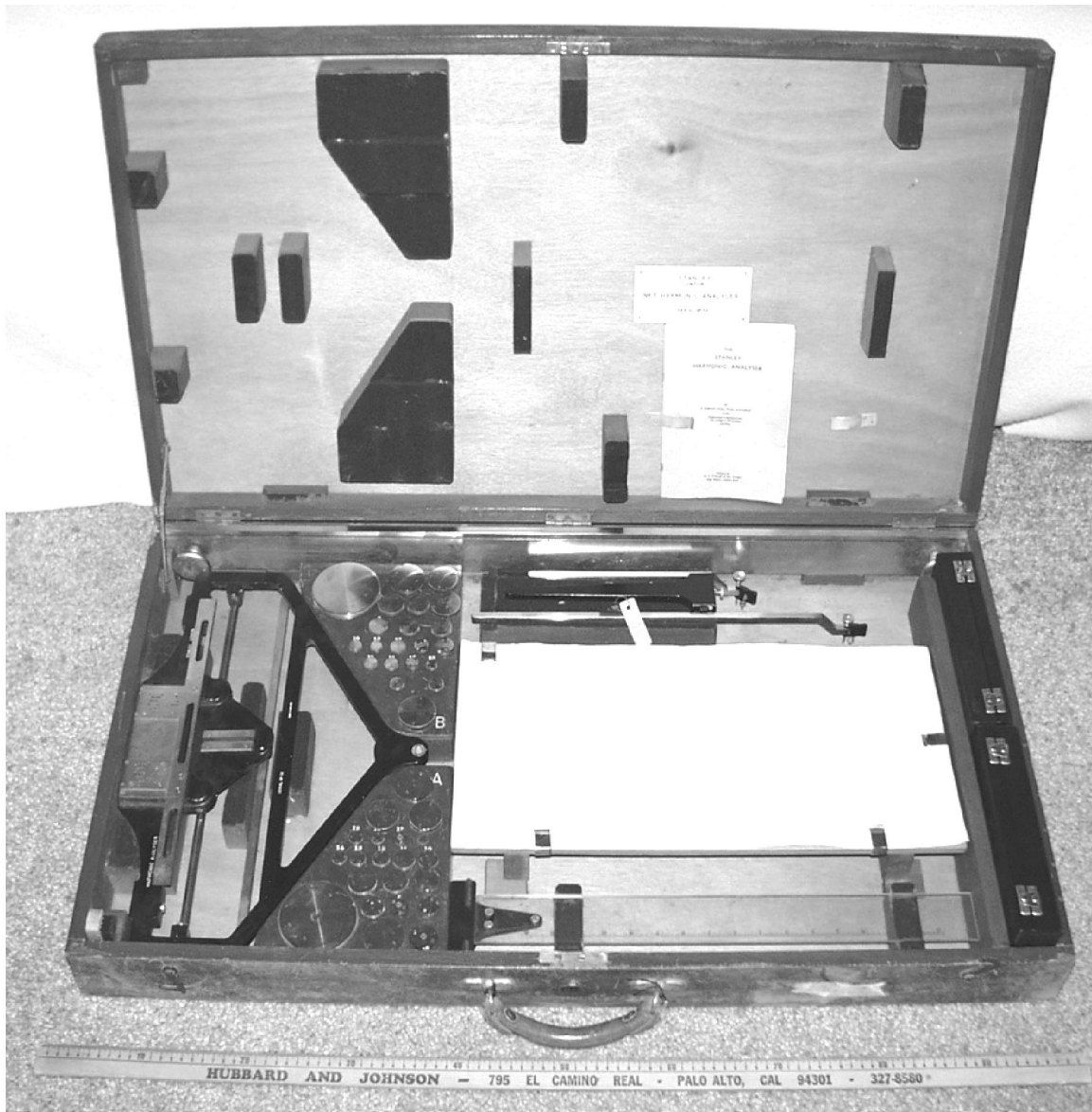
Figure 7b. The Yule, Mader, Ott analyzer, as made by W.F. Stanley. 4 It processes 18 harmonics.
