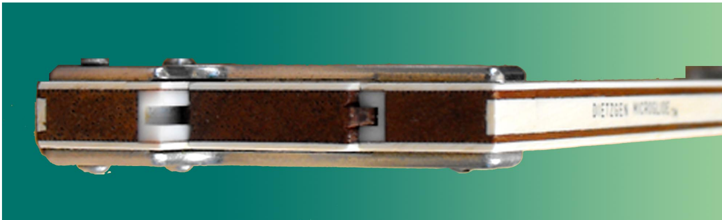
FIGURE 4. Teflon Inserts in the Microglide duplex.
