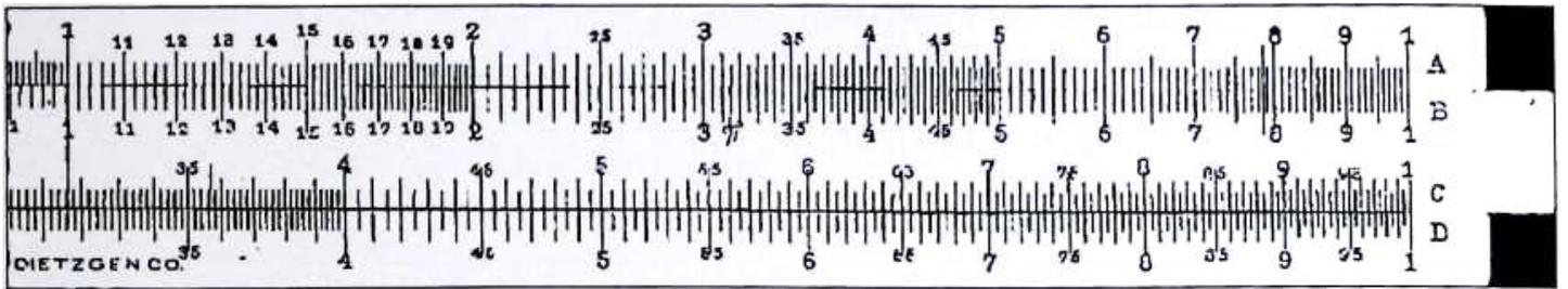
Figure 4.6.1.1.5.R: Right part of the front of the Rosenthal system from Dietzgen. Rodger Shepherd collection
