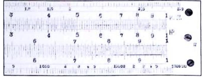
Figure 3.6.1.5.R: Right part of Schweth's Electro slide rule
