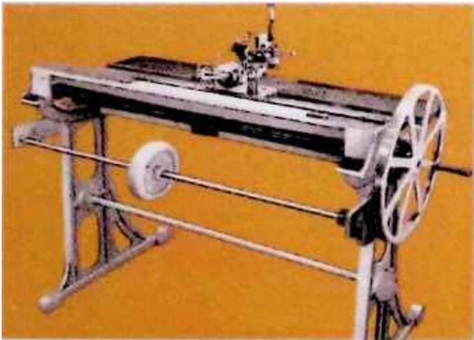
Figure 4.1: First dividing machine from D&P
