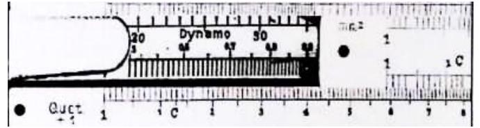
Figure 3.8.1.5.L: Left part of the Faber electro slide rule
