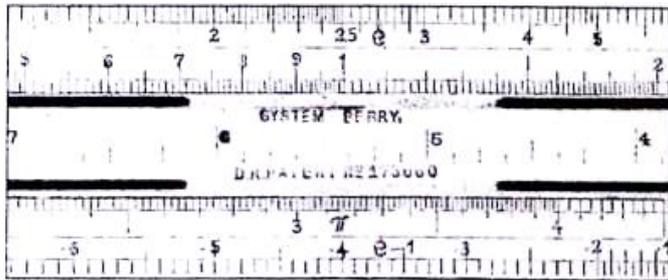
Figure 4.5.3.4: Perry System with *D.R. Patent 173 660*
