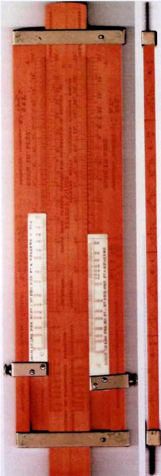
The front has 10 scales; the reverse (not shown) has 6 scales and a table. Despite the many scales and supporting texts, the staff is very clearly designed.
