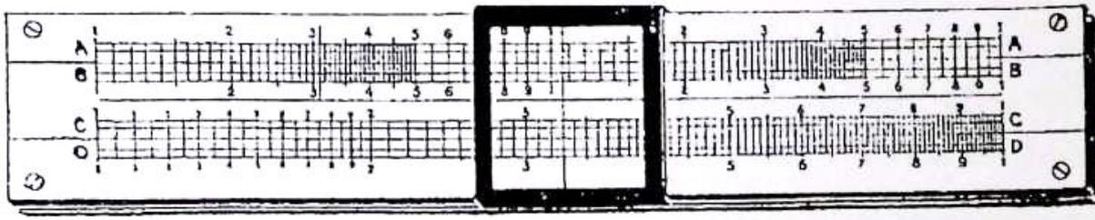
Figure 4.3.6.1: 1903 system Simplex pocket slide rule with screws. Journal of Surveying
