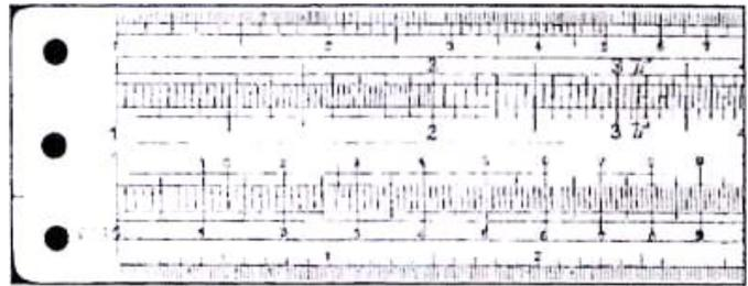
Figure 4.4.4: Slide rule System Rietz
