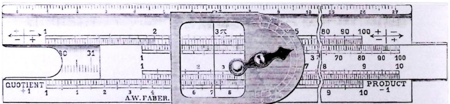
Figure 3.8.1.1: Direct marking of the number of digits by means of inscriptions and marks
