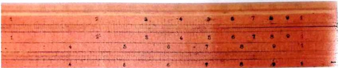
Figure 3.4.3.R: Right part of the front of the Mannheim system by Tavernier-Gravet
