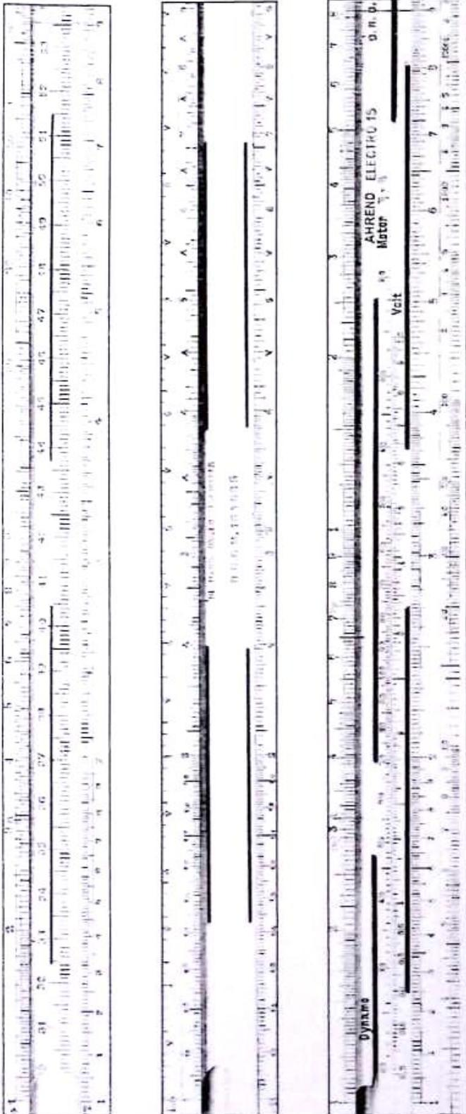
Figure 6.7: Slide rules with 2, 4 and 5 slots
