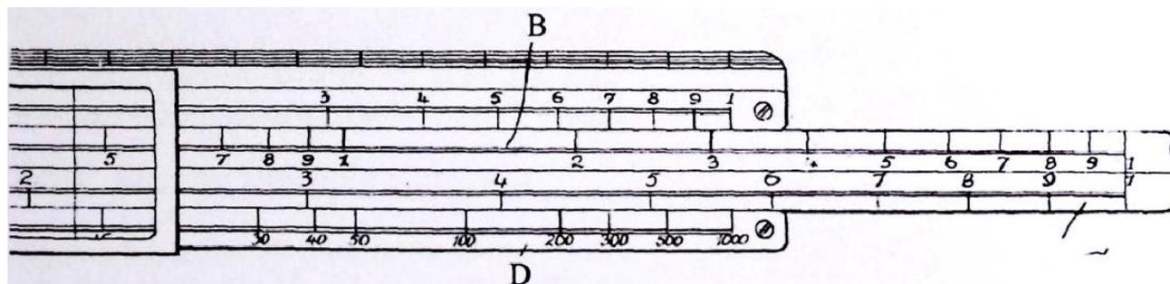
Figure 4.5.3.2.R: Right part of the drawing of Perry's prototype
