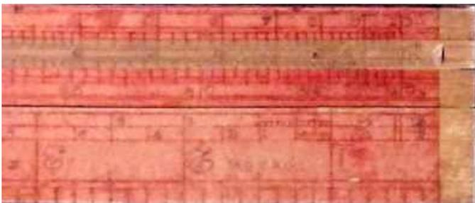
Figure 6.11.3: Section of the Coggeshall system
