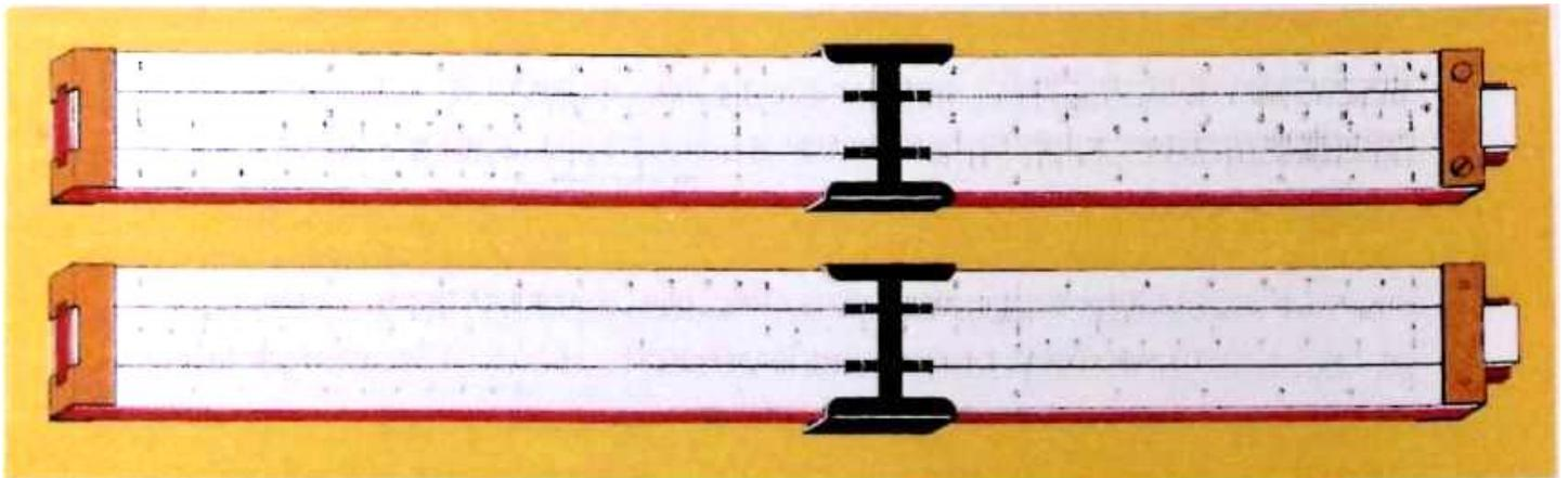
Figure 4.1.2: Two-sided slide rule by William Cox, manufactured by D&P
