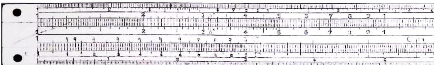
Figure 3.9.4.L: Left part of the front of the narrow version of the Rietz system from Nestler (25 instead of 31mm)
