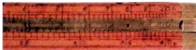
Figure 3.1.2: Section of the Coggeshall system
