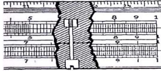
Figure 4.3.5.1: Position of the adjustment screws
