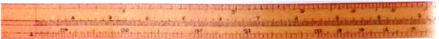
Figure 3.4.4.L: Left part of the back of the slide of the Mannheim system by Tavernier-Gravet
