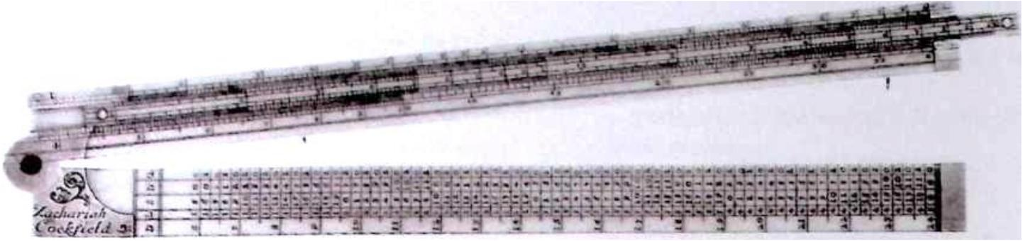
Figure 6.11.1: Coggeshall system with rail-shaped scales, manufactured by Edmund Culpeper at the beginning of the 18th century
