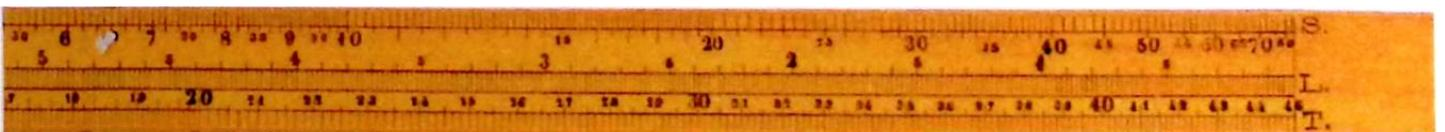
Figure 3.8.1.4.R: Right part of the back of the slide of the Mannheim system by A. W. Faber. Werner Rudowski collection
