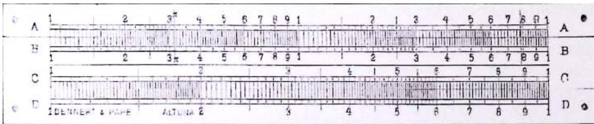
Figure 4.3.6.3: System Simplex pocket slide rule with rivets. IJzebrand Schuitema collection
