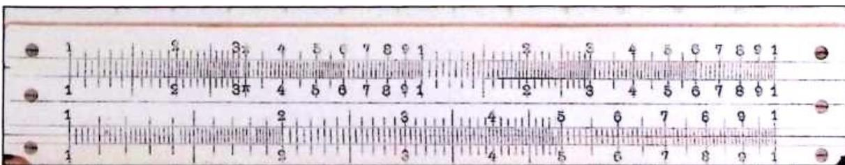
Figure 3.6.2.4: Tavernier-Gravet's slide rule from 1925 with celluloid veneer and *longitudinal lines* (see p.36).
