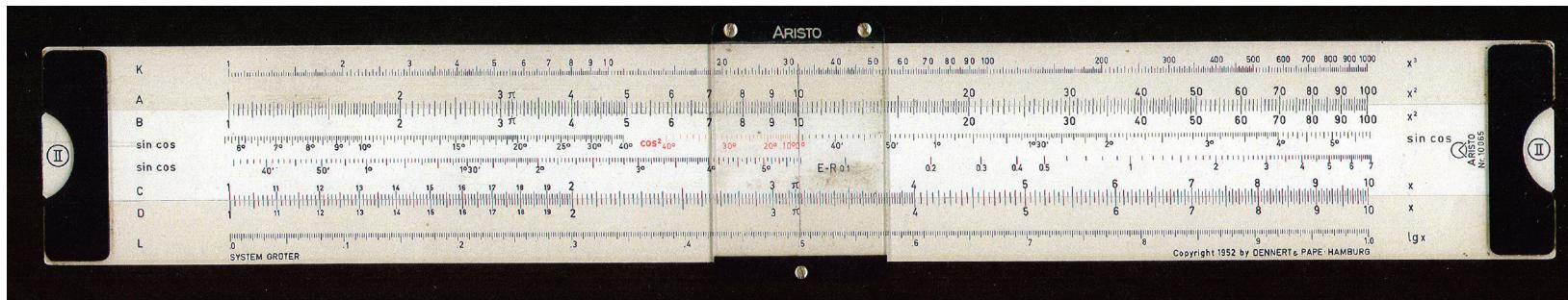
Note the E-R scale; for correcting the vertical height, V, due to the earths curvature and refraction
