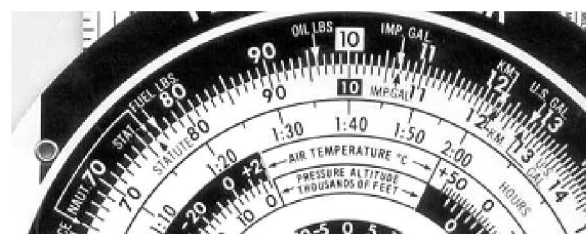
Figure 11. Conversion Gauge Marks on E6B.
