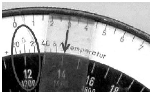
Figure 15. True Airspeed Calculation on DR2.
