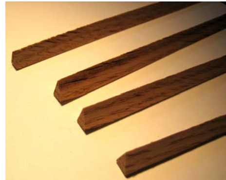
FIGURE 5. Triangular bars \frac{3}{8} \times \frac{1}{4} \times \frac{3}{8} inches
