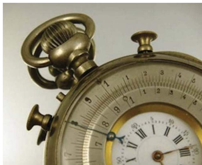
FIGURE 4. Detail of the Slide Rule and Ring-Mounted Cursor 4
