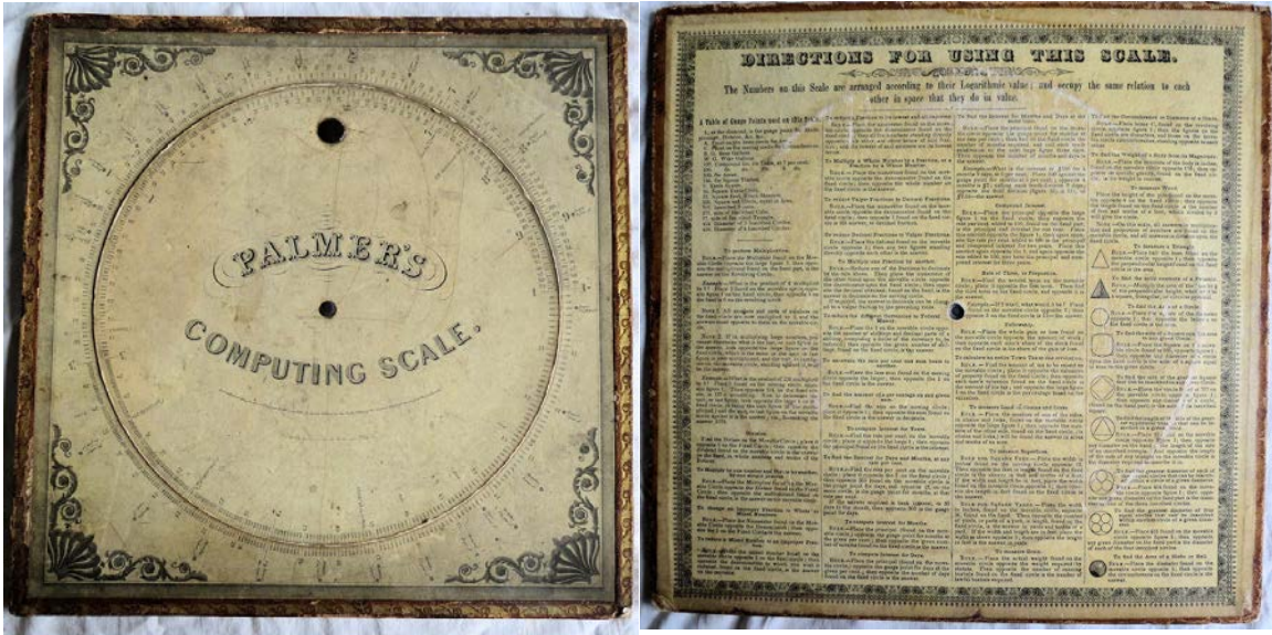
1843 Palmer's Computing Scale, Lithographed Circular Slide Rule, one of the earliest production circular slide rules made in the US, c.1850. Rare version with instructions on the reverse. Gauge marks for geometry, timber, excise, physics, accounting, etc. calculations. Sold for just $138.
