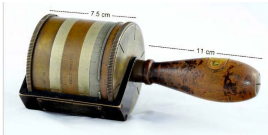
Barr & Stroud Inclinometer, Survey & Artillery Type S.L.2 No 58, Slide Rule Most interesting cylindrical slide rule with special scale set for determining slope angle to a distant site. Made of copper, brass, aluminum and oak. Note that this instrument has a wood handle like a Fuller Calculator, but instead of spiral scales, it has 3 separate ring scales and one pointer scale. $234
