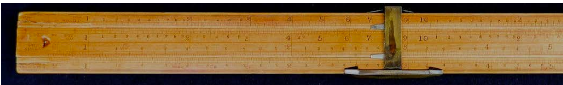
Stanley, Froude's Ship Displacement Slide Rule, 24" Boxwood with Chisel Cursor. Has scales for Hull Displacement, Weight & Length, Horse Power & Speed. See UK Slide Rule Gazette, Issue 3, for more details. Two sold for $195 & $225
