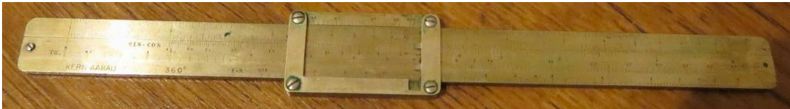
Kern AARAU Surveyor's Slide Rule, 25-cm Metal Body & Metal Chisel Cursor. With Sin*Cos, TG, E*R Scales on Body and Angle Scale on Cursor, Swiss Made. $208
